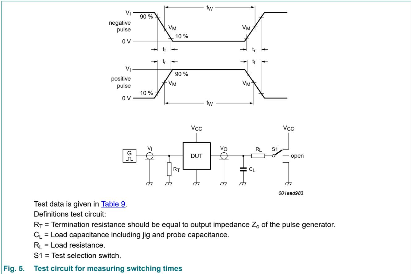
Fig. 5. Test circuit for measuring switching times
